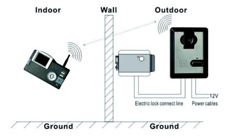
After pressing the Unlock key of the monitor, it transfers the singal of unlock to the camera in the way of wireless, and the E-lock will be opened(electronic lock connected with the camera by electronic cable)
